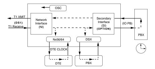
Figure 5-6. Secondary Timing
